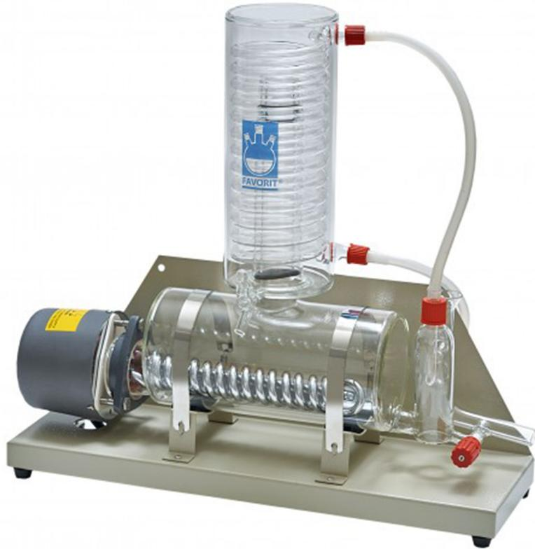
Horizontal thick wall heat resistant borosilicate glass boiler fitted with 3 KW chromium plated heater.
